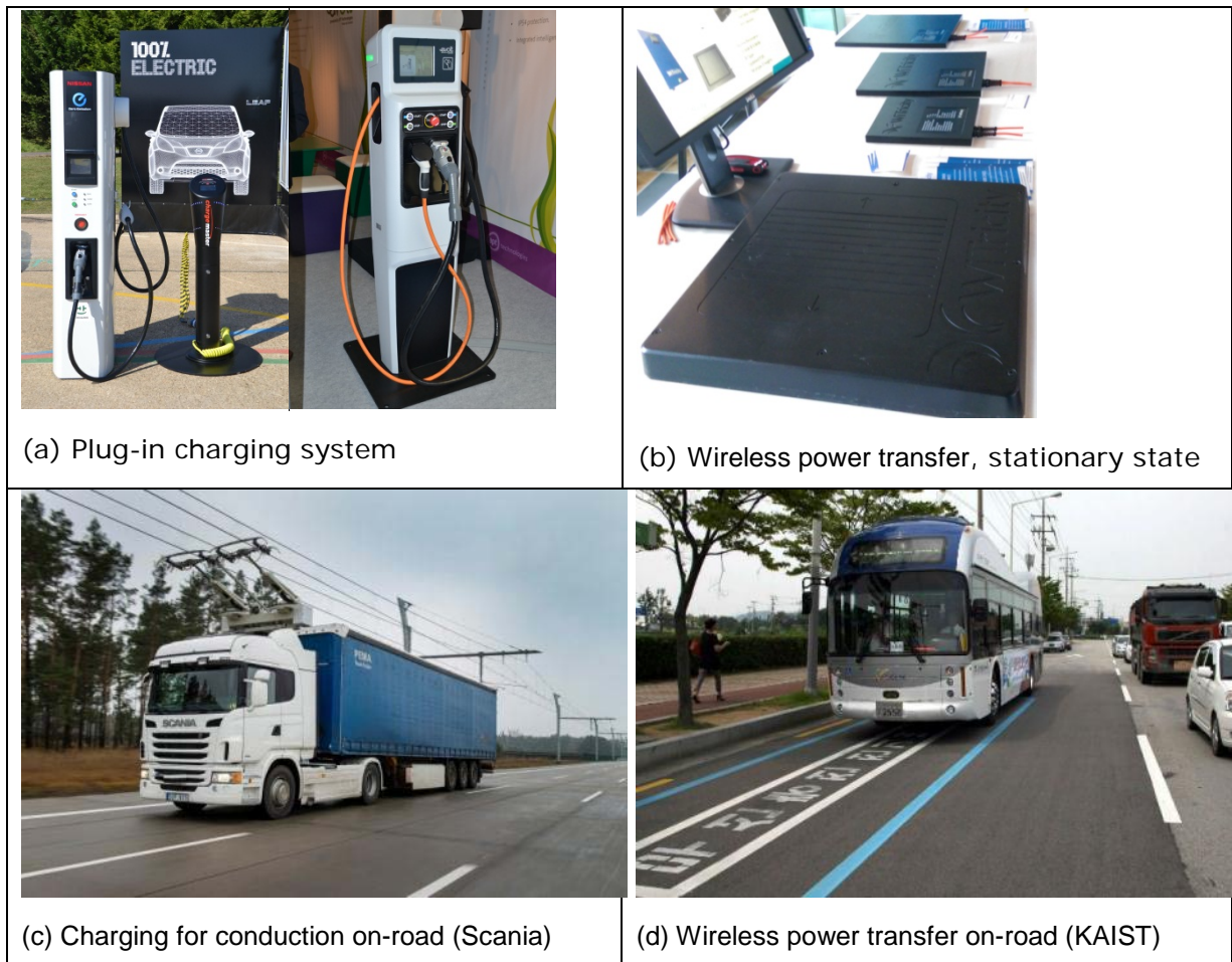
Figure 8: Types of power transfer solutions
