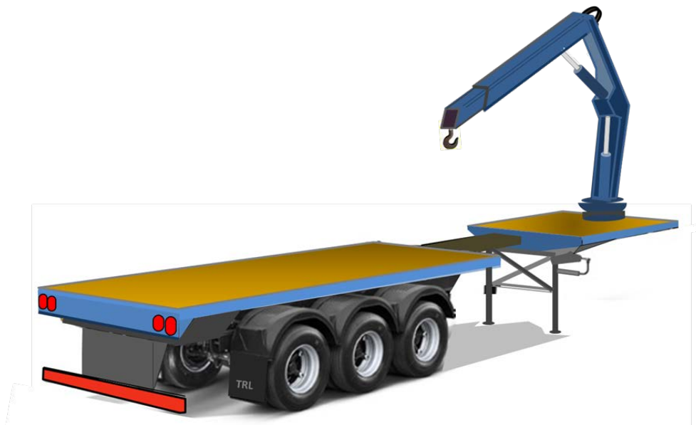
Figure 26: Example of extendible trailer that could be used for prefabricated sections installation
