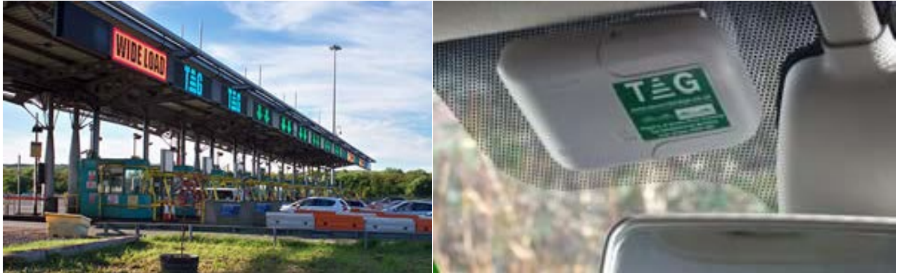
Figure 43: Second Severn Crossing TAG system Toll sensors and in car TAG unit
