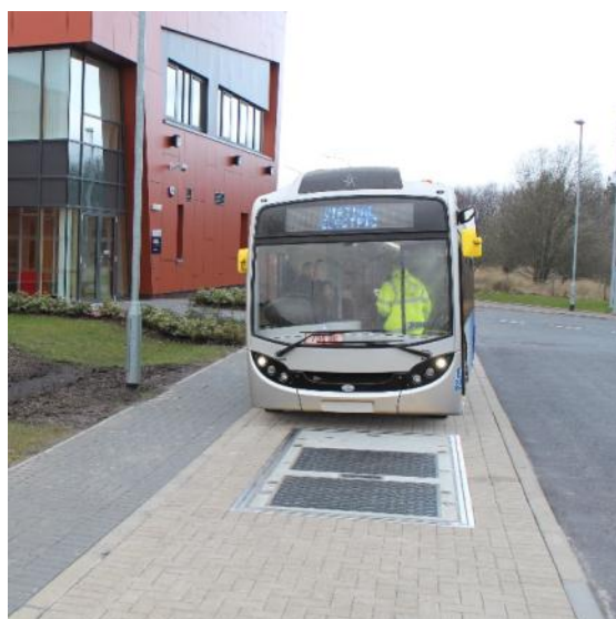
Figure 16: IPT Technology chargers trialled in Glasgow
